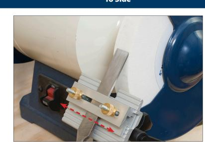
The slot assembly allows you to remove your tool from the platform for checking your progress. Once you have checked your tool you can go right back to sharpening without loosing your angle or make necessary adjustments on the fly.
